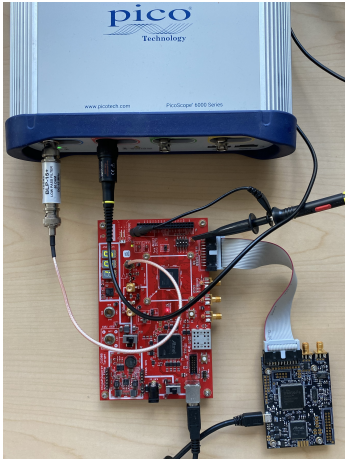
Fig. 7: Experimental setup for capturing power traces.
