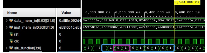
Figure 8: Simulation of the alu_func register during the computation of one neuron in the last layer (blue: the execution window of one neuron; purple: the execution window of one multiplication and summation corresponding to each connected input).
