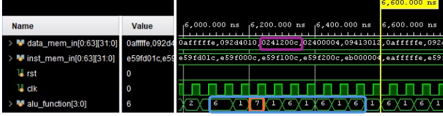
Figure 9: Simulation of the alu_func register during the computation of one neuron in the last layer after fault injection (blue: the execution window of one neuron, purple: the changed data register value due to the fault injection, orange: the value of the alu_func after fault injection).
