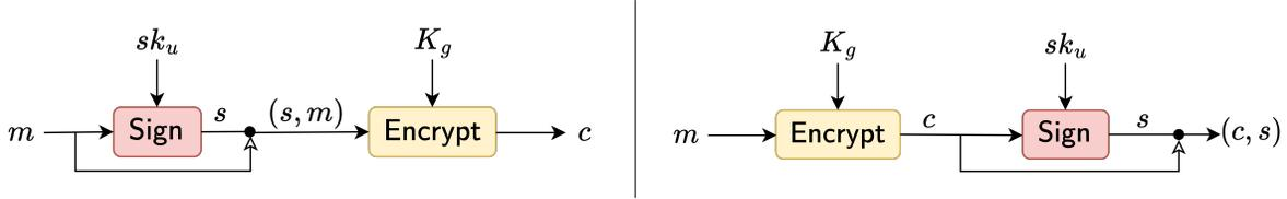
Fig. 1: Warmup schemes obtained by composing digital signatures with symmetric encryption. **Left pane:** Sign-then-Encrypt. **Right pane:** Encrypt-then-Sign.
