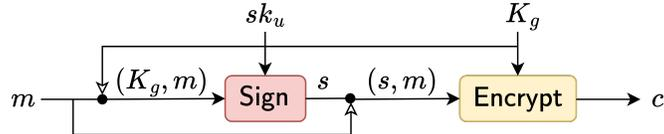
Fig. 2: A high-level representation of the SealPacket scheme in Keybase.
