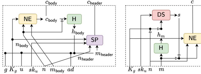
Fig. 13: The BoxMessage/BM (Left) and SealPacket/SP (Right) algorithms used to encrypt chat messages and message headers in Keybase. We omit the inputs  $g$ ,  $u$ , and  $ad$  from SP as it does not use  $g$  or  $u$  and  $ad = \varepsilon$  always holds.
