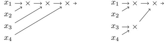
Figure 3. Two circuits that compute  $x_1 \times x_2 \times x_3 \times x_4$ . Left, an inefficient circuit of depth 3. Right, an optimal circuit that uses a binary tree to compute the product in depth 2.
