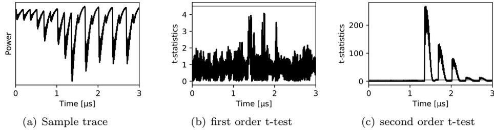
**Figure 7:** Case study 2: fixed-vs-random t-test results for the ANDXOR4 experiment (100M traces) with LFSR8\_X4 as source of fresh randomness.
