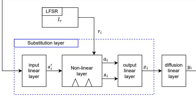
**Figure 4:** Top-level representation of the Ascon permutation.
