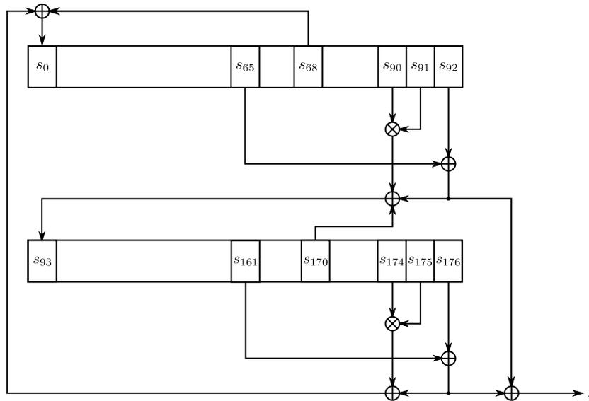
**Figure 2:** Schematic of Bivium B, a reduced security variant of the stream cipher Trivium consisting of 2 NLFSRs.
