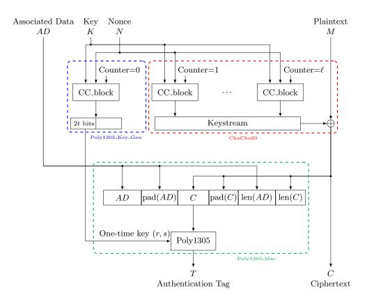
Fig. 4. The encryption procedure in ChaCha20-Poly1305.
