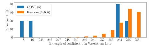
Fig. 6: Two GOST curves (CryptoPro-A-ParamSet, CryptoPro-C-ParamSet) exhibit particularly low bit-length of b parameter, even though Alekseev, Nikolaev, and Smyshlyaev [ANS18] claim that they were generated pseudorandomly.
