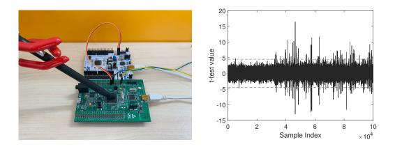
Figure 4: Our SCA equipment (left) and TVLA results between re-encryption of  $m_0$  and  $m_1$  (right)
