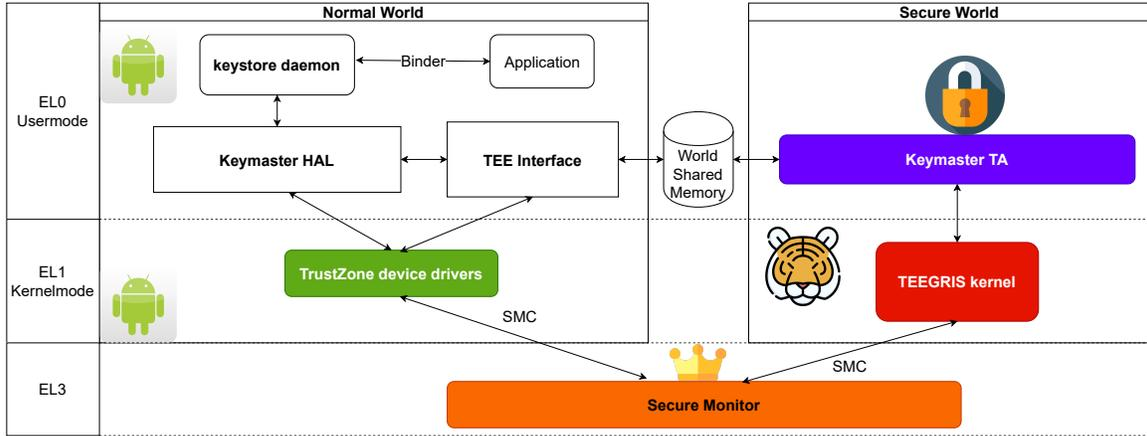
Figure 3: Overview of the Hardware backed keystore<sup>2</sup>
