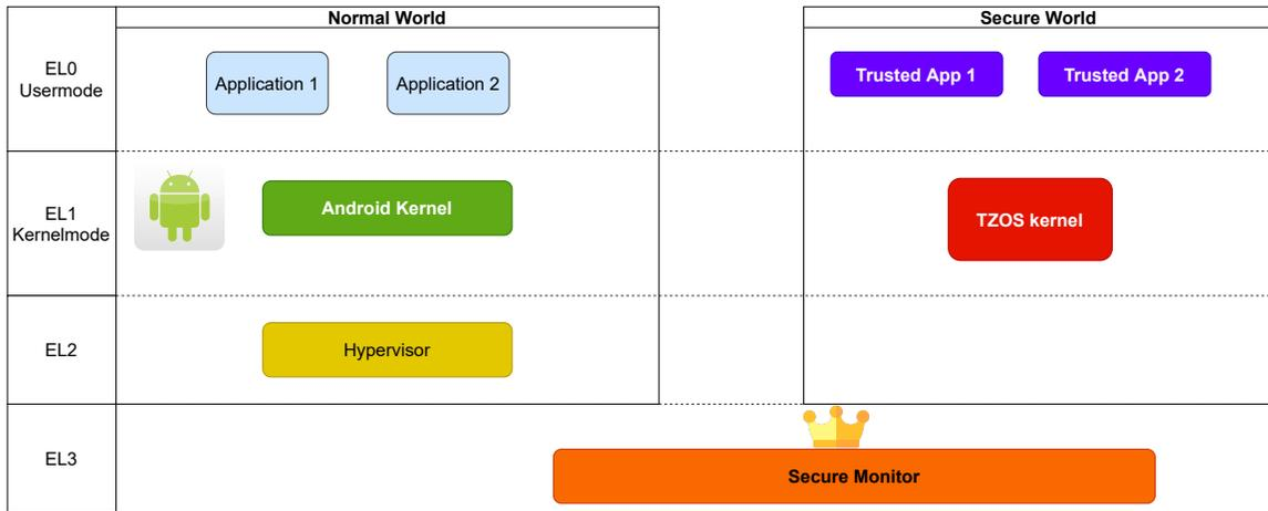
Figure 1: The TrustZone software and hardware isolation architecture <sup>2</sup>
