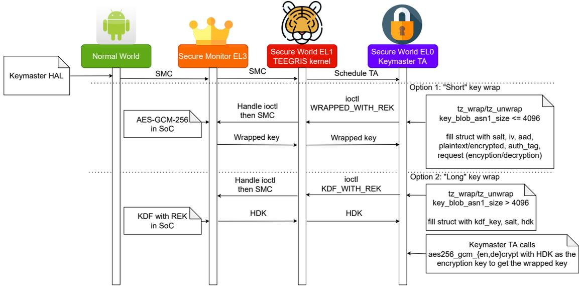
Figure 8: Key wrapping in Keymaster TA in TEEGRIS <sup>2</sup>
