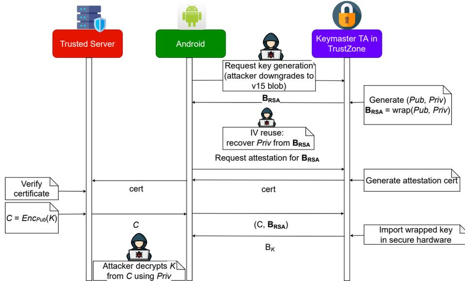
Figure 5: Simplified Secure Key Import: the “hacker” icons indicate the interception points used in our attack <sup>2</sup>
