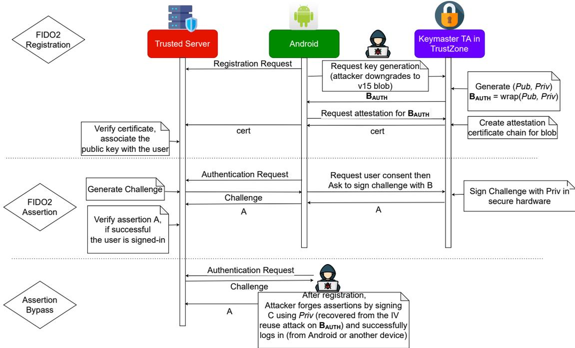
Figure 6: FIDO2 WebAuthn: the “hacker” icons indicate the interception points used in our attack <sup>2</sup>
