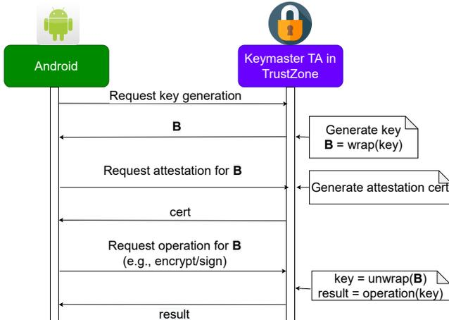
Figure 2: A usage example of an Android application using a Hardware-Backed Keystore (i.e., the Keymaster TA) for cryptographic key management: key generation, attestation, and encryption/signature.<sup>2</sup>
