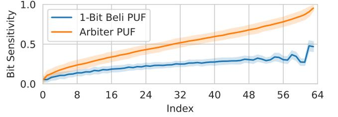
Fig. 4. Probability that flipping the input bit at the given index will change the PUF’s output bit, as empirically estimated for 1-bit Beli PUF and Arbiter PUF. Estimations are based on 100 simulated instances, where the probability for each index was approximated using 1000 uniform random noise-free challenges. The shaded area indicates the standard deviation interval of the bit sensitivity.
