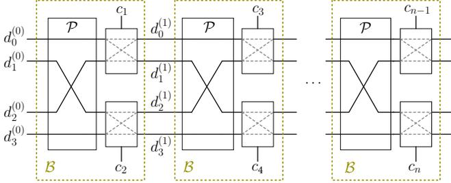
Fig. 1. Beli PUF structure. Permutation network of the Beli PUF. TODO change from 0-index to 1-index
