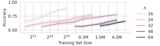
Fig. 5. Prediction accuracy of a general-purpose MLP modeling attack on 1-bit Beli PUF, simulated with various challenge sizes for 10 instances using noise-free CRP data sets of size  $N$ . The shaded area indicates a 95% confidence interval across attacked PUF instances.
