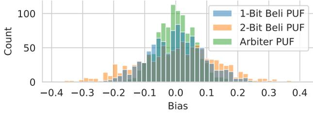
Fig. 3. Distribution of the bias of 1-bit Beli PUF, 2-bit Beli PUF, and Arbiter PUF for 1000 instances each. Each bias has been estimated by querying 1000 uniform random, noise-free challenges.
