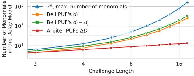
Fig. 2. Number of monomials for the Beli PUF’s  $d_0$ ,  $d_1$  and their difference  $d_0 - d_1$ , as well as for the Arbiter PUF delay model, when written as multivariate polynomial of the challenge.
