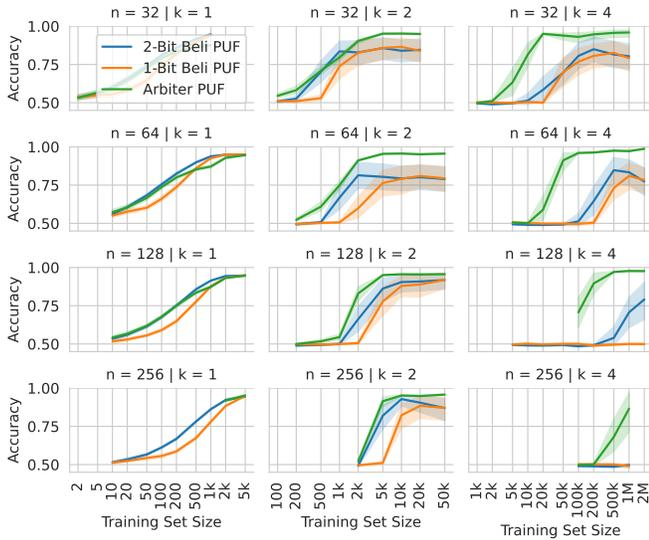
Fig. 6. Accuracy obtained when attacking the 1-bit Beli PUF, 2-bit Beli PUF, and XOR APUF. For each combination of challenge length  $n$ , number of CRPs  $N$ , number of XORs  $k$ , and PUF type, we ran at least 10 attacks with individual PUF simulation and attack initialization each. The accuracy shown is evaluated on an independent 1,000 CRPs test set. The shaded area indicates a 95% confidence interval across attacked PUF instances.
