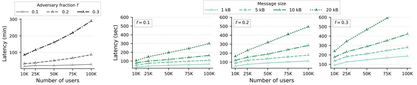
**Figure 8:** **Left:** Path establishment with different fractions of malicious servers ( $f$ ). **Right:** Broadcast round scaling with number of users  $M$  (messages), message sizes, and different adversary fractions. Both experiments are run on a simulated 200 Mbps network configuration with  $N = 128$  servers. Shaded regions represent a 95% confidence interval (mostly invisible).
