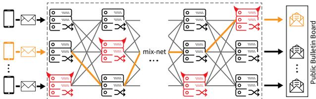
**Figure 1:** Trellis arranges the set of servers into “layers,” (each server appears once per layer) to instantiate a mix-net. Users send messages through a random path which guarantees that all messages are mixed before reaching the public bulletin board, even when a subset of servers are malicious (colored in red).
