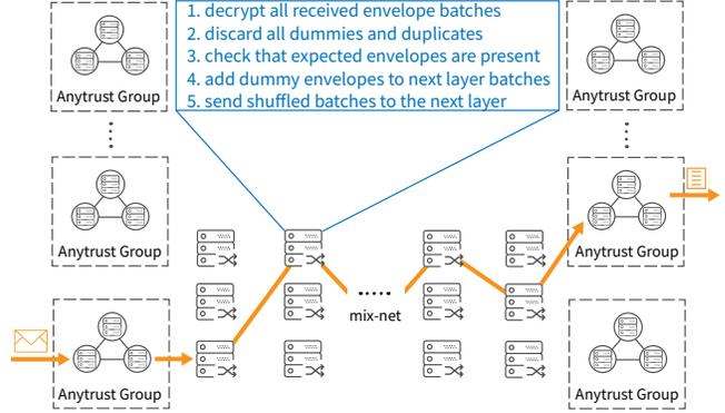
**Figure 6:** Detailed overview of the Trellis mix-net “book-ended” by anytrust groups to prevent denial-of-service attacks at the entry and exit points. Users send boomerang-encrypted messages through a pre-selected random path in the network. The anytrust group at the last layer ensures that all messages get published to the bulletin board.
