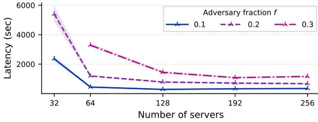
**Figure 9:** Latency decreases with the number of servers added to the network (until reaching a constant overhead) with 200 Mbps bandwidth cap. Number of messages is  $M = 2,000,000$  and message size is set to 1 kB. Shaded regions represent a 95% confidence interval.
