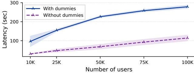
**Figure 10:** Dummy envelopes between layers incur a large overhead due to increased bandwidth requirements. Broadcast round (with and without dummy envelopes) evaluated on the real network with 200Mbps bandwidth cap,  $f = 0.2$ , and message size set to 10 kB. Shaded regions represent a 95% confidence interval.
