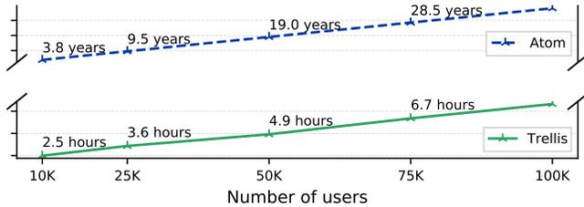
**Figure 11:** Latency of Trellis vs. Atom to broadcast a 1 MB file. We vary the number of users and set  $f = 0.2$  for both systems (we run Atom on 32 B messages and extrapolate) with 200 Mbps bandwidth cap.
