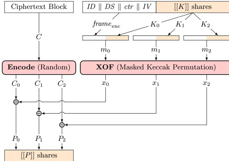
**Fig. 1.** The  $\text{WrapQ}^{-1}$  key import function uses a masked XOF in counter mode to decrypt ciphertext blocks  $C$  into randomized Boolean shares  $[[P]]$ . The Keccak Permutation (pictured here with three shares) exists in secure implementations of Dilithium and Kyber; WrapQ just reuses the component.
