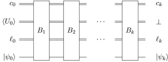
Figure 3:  $M$ -qubit quantum computation with classical post-processing. Each block  $B_i$  corresponds to the circuit in Figure 2 with the corresponding choices of input and classical post-processing  $f_i$ .
