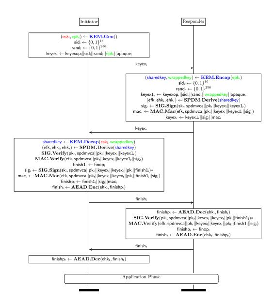
Fig. 3. PQ- SPDM KEM-based key exchange flow
