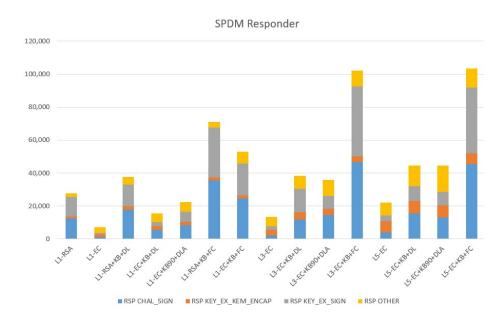
Fig. 7. SPDM responder performance - Kyber, DILITHIUM, FALCON (microsecond).
