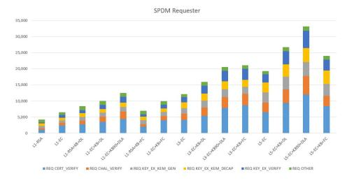
Fig. 5. SPDM requester performance - Kyber, DILITHIUM, FALCON (microsecond).
