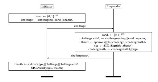
Fig. 1. SPDM device authentication flow.
