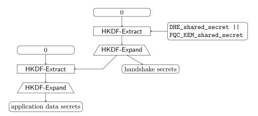
Fig. 4. SPDM key derivation flow.
