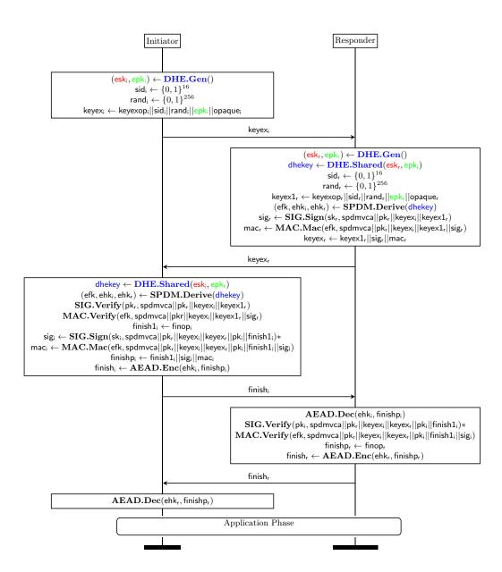
Fig. 2. Traditional SPDM DHE-based key exchange flow.
