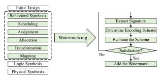
Fig. 5: A generic approach for watermark insertion at the behavioral synthesis level [26].
