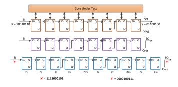
Fig. 10: DFT-based watermarking scheme [15].
