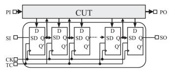
Fig. 9: Scan chain design used in DFT [15].
