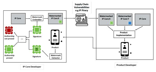
Fig. 1: IP watermarking embedding and verification.
