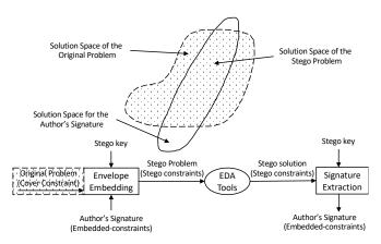
Fig. 3: Basic concept of the constraint-based watermarking approach [41].
