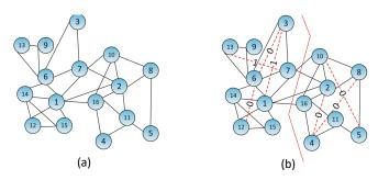
Fig. 4: (a) Graph to be partitioned with nodes indexed by integers (b) The partitioned graph with embedded watermark [43].
