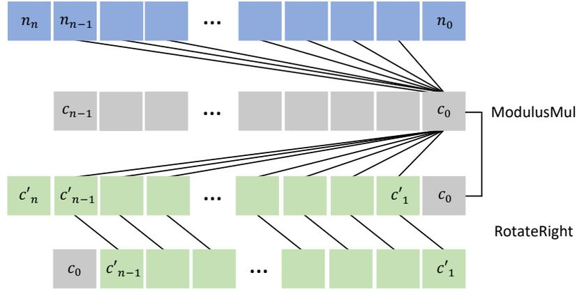
Fig. 2: ModulusMul + RotateRight.
