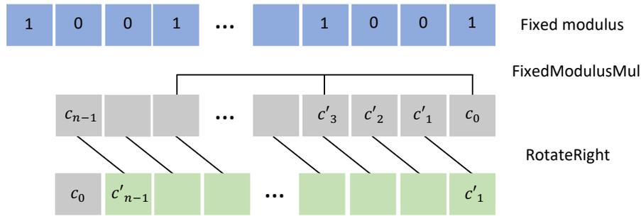
Fig. 4: FixedModulusMul + RotateRight.
