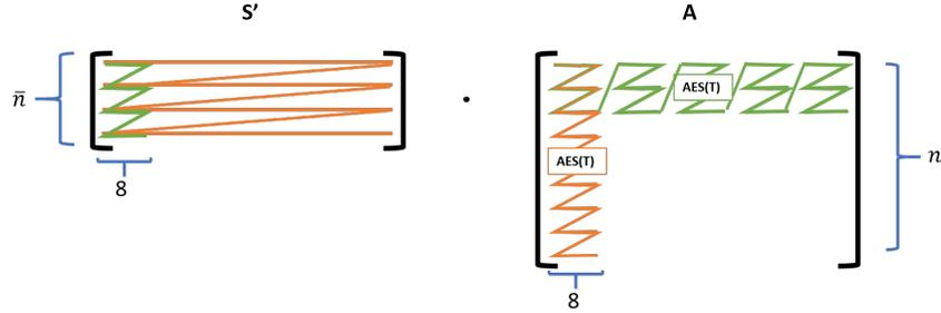
**Fig. 1.** Graphical representation of processing the elements. In orange the FrodoKEM approach, which for cache-friendly access requires transposing the blocks of columns from  $\mathbf{A}$ , before multiplying with the rows of  $\mathbf{S}$ . In green the RWCF approach, which does not require a transpose.
