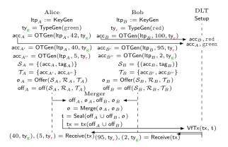
Fig. 2. Example of a full SwapCT system with setup, type registration and an atomic swap of 2 green for 5 red tokens between Alice and Bob with an untrusted Merger and DLT. Sampling of the rings  $\mathcal{R}_a$  and  $\mathcal{R}_b$  is covered by related research [16].
