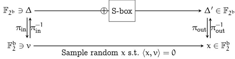
Figure 4: Subtracting Key followed by S-box  $\approx$  Subspace Sampling, modulo Change of Variables
