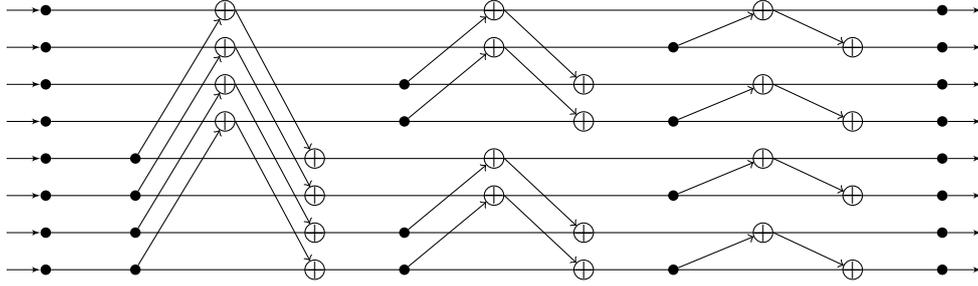
**Figure 4:** The three stages of butterflies in a size-8 AFFT. Each arrow going upwards is associated with a constant which is not shown, so it actually means “adding the product of the source and the constant to the destination” instead of “adding the source to the destination”.
