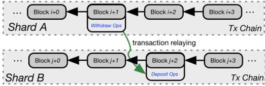
Fig. 2: Message passing mechanism across distinct shards with the help of relay transactions based on *Account/Balance* model.
