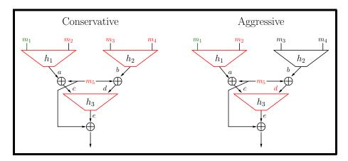
Fig. 3. Conservative and aggressive openings for  $T_5$ . Green  $m_1$  is opened. Red are opening elements (4 vs 3) and recomputed compression functions (3 vs 2).
