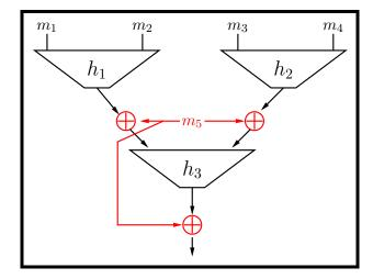
Fig. 1. The  $T_5$  construction with five message blocks  $m_1, m_2, m_3, m_4, m_5$  and three compression function calls.
