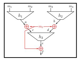
Fig. 2. Modified 2-level Merkle tree  $T_5(m_1, m_2, m_3, m_4, m_5)$  with an extra input  $m_5$  for the same 3 hash calls.
