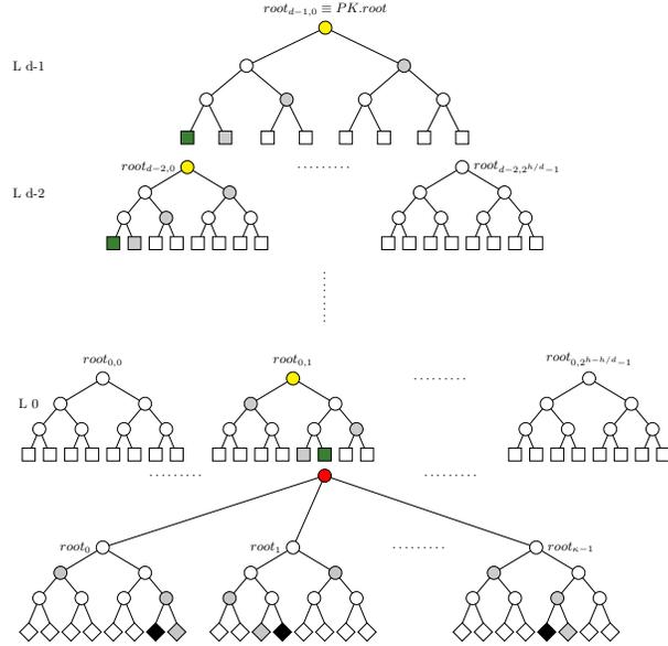
Fig. 1: Simplified SPHINCS<sup>+</sup> depiction where the FORS trees and subtrees are 3 levels high. The diamond, circle, and square nodes denote FORS leaves, intermediate hash nodes, and WOTS<sup>+</sup> leaves, respectively.
