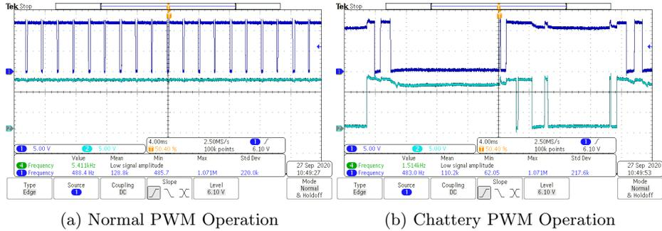
Fig. 7: PWM output for throttle body control before and after EMFI insertion.
