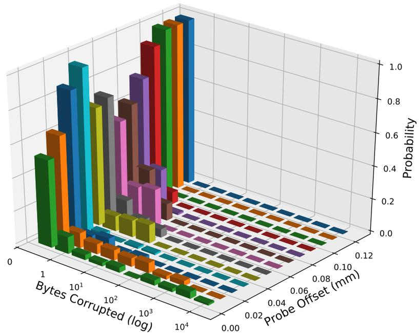
Fig. 4: Changing the distance from the SRAM surface causes a differing number of faults to occur.
