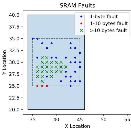
Fig. 5: SRAM Fault Results (200V), light blue is SRAM chip top, dashed area shows scan zone.
