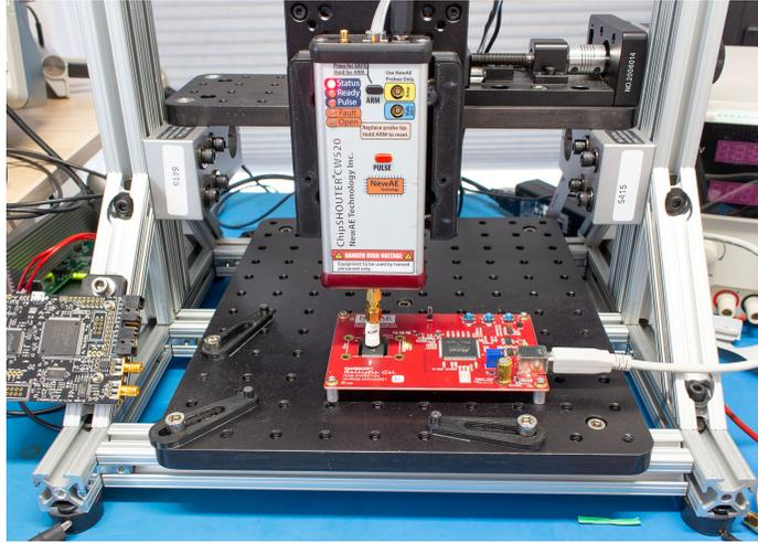
Fig. 1: Ballistic Gel mounted on XYZ table with EMFI Tool
