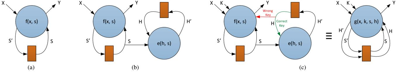
Fig. 1: Logic encryption scheme (a) Original circuit (b) Structural transformation (c) Sequential encryption
