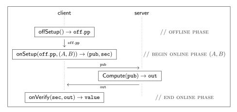
Fig. 1. Diagram visualizing the model for offline/online pairing delegation. Notably, the pairing arguments (A, B) are revealed only at the start of the online phase. The one-time GlobalSetup is omitted from the picture.
