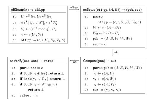
Fig. 2. Di Crescenzo et al.'s protocol for secure pairing delegation with online public inputs (see Section 3 in [21]). This description uses a different, more intuitive notation. The GlobalSetup is not included explicitly as it is trivial.
