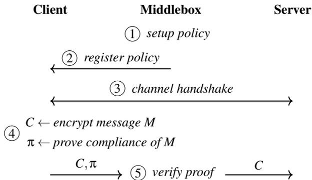
Figure 1: Structure of our ZKMB protocol. The client convinces the middlebox that the message  $M$  is policy-compliant without revealing it. The handshake and encryption algorithms are part of the underlying secure channel (such as TLS). Transcripts and secrets generated in the handshake may be inputs to the proving and verification steps.
