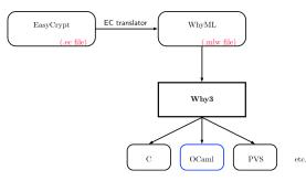
Fig. 19: EasyCrypt extraction tool-chain. We only extract OCaml code in this work, but there are resources online suggesting that C and PVS code could also be extracted from WhyML.
