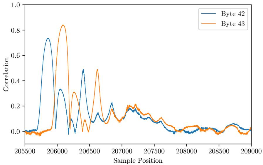
(b) HW leakage of bytes 42 and 43
