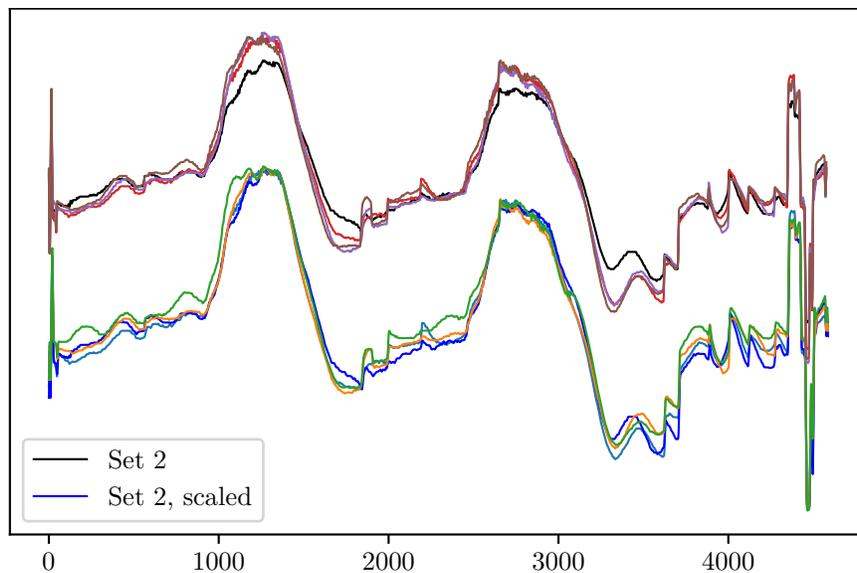
**Fig. 5.** Selected trace indices at byte position 43 with hamming weight 4 before (top) and after (below) min-max row normalization. The traces after applying normalization were additionally shifted down along the y-axis for this illustration.
