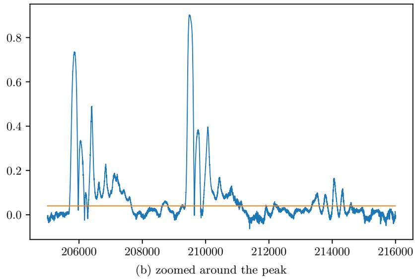
**Fig. 6.** Correlation points of interest w.r.t. key byte position 42 of the key expansion. The orange line indicates a threshold of 0.04.
