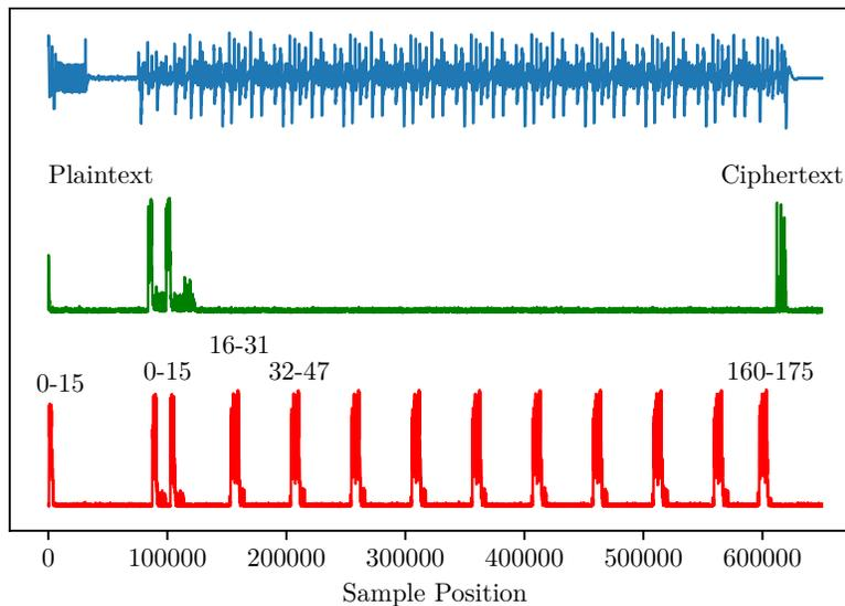
**Fig. 1.** Full mean trace of Set 3 (blue), detected plaintext and ciphertext leakage (green) as well as key expansion leakage grouped as complete AES-128 round keys (red). Leakage is computed using CPOI.
