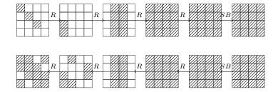
Fig. 5. 5-round truncated differential characteristic used in key recovery attack AES
