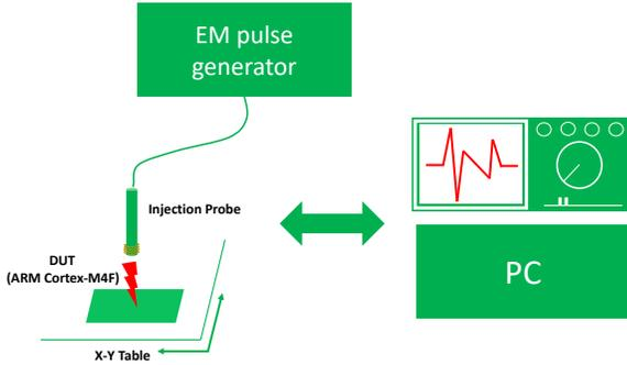
Figure 2: Experimental setup for the fault injection
