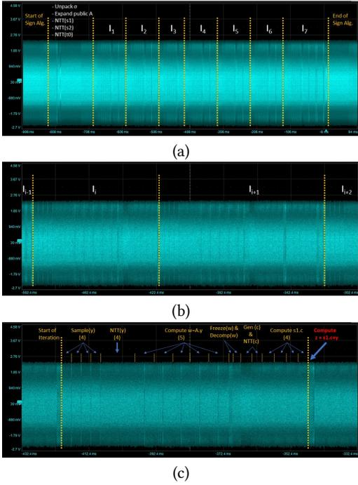
**Figure 8: First order Pattern Recognition (a) Identification of multiple iterations of signing procedure on EM trace (b) Zoomed in view of multiple iterations (c) Identifying repeating patterns in a single iteration and mapping them to the corresponding operations in the reference implementation**
