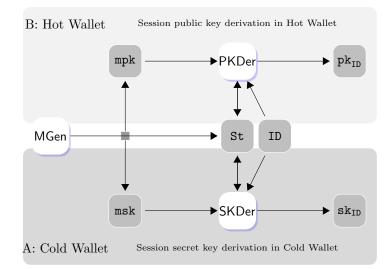
Figure 3: Both Hot/ Cold wallet internally stores the common state St. The master keys are stored in the respective wallets. When a session secret key is generated within the cold wallet as  $(sk_{ID}, St) \leftarrow$ SWal.SKDer(msk, ID, St), the state St gets refreshed. The session public key  $pk_{ID}$  is generated within the hot wallet as  $(pk_{ID}, St) \leftarrow$  SWal.PKDer(mpk, ID, St), and the corresponding state St is refreshed in the same manner.
