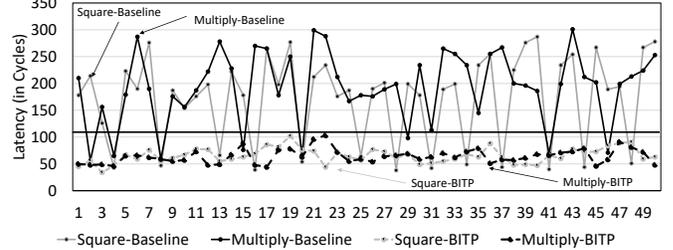
Fig. 4. LLC access time observed by the attacker while attacking GnuPG. Y-axis shows LLC access time. X-axis: attack epochs.
