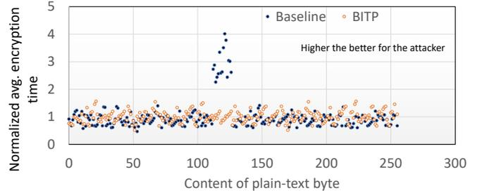
Fig. 3. Normalized average encryption time observed by the attacker for different plain-text values on AES-128. Higher avg. encryption time leads to a successful Evict+Time attack.
