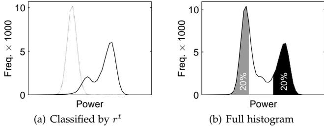
Fig. 3. SCA of the top layer of original (1, 5)-IPUF using 100 000 averaged signals, histograms at the point of interest identified in Figure 2(b).
