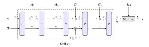
Fig. 10: Graphical illustration of SLMAC- $\mathcal{T}$ .
