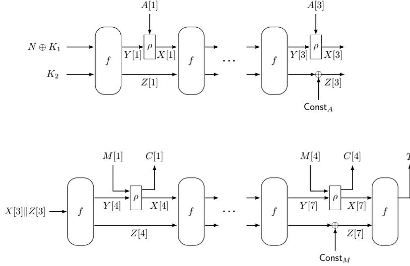
**Figure 1:** Beetle Construction with  $a = 3$  associated data blocks and  $m = 4$  message blocks. The value  $\text{Const}_A$  and  $\text{Const}_M$  is used to denote whether last associated data block and message block is complete or not.
