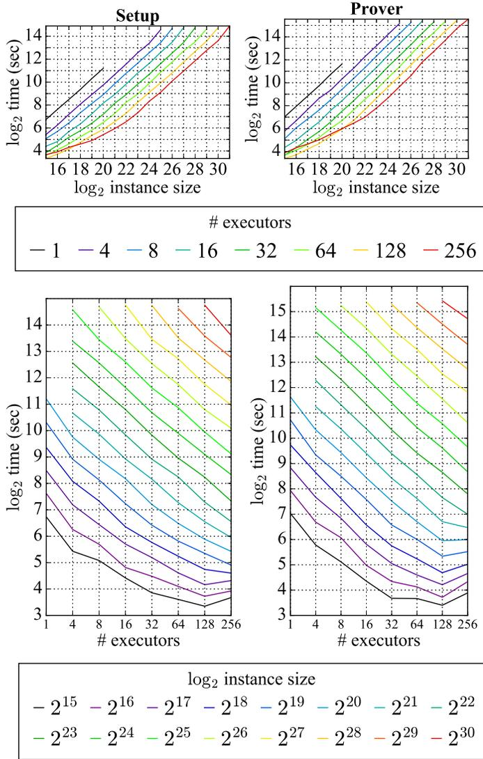
**Figure 7:** Setup and prover running times for different combinations of instance size and number of executors.
