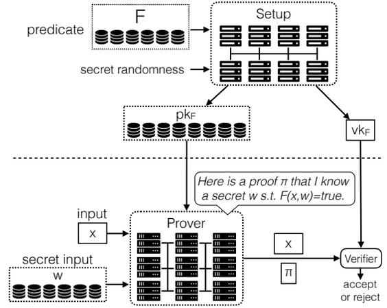
**Figure 3:** A distributed zkSNARK. The setup algorithm is run on a compute cluster, and generates a long proving key  $pk$ , held in distributed storage, and a short verification key  $vk$ . The prover algorithm is also run on a compute cluster.
