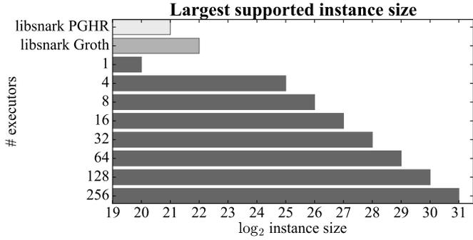
**Figure 6:** Largest instance size supported by `libsark`'s serial implementation of PGHR's protocol [PGHR13] and Groth's protocol [Gro16] vs. our distributed system.
