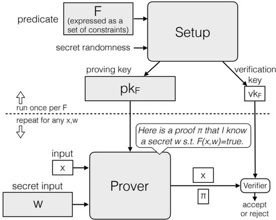
**Figure 2:** Components of a zkSNARK. Shaded components are those that we distribute so to support proving/verifying statements about large computations. Prior systems run these as monolithic procedures on a single machine.
