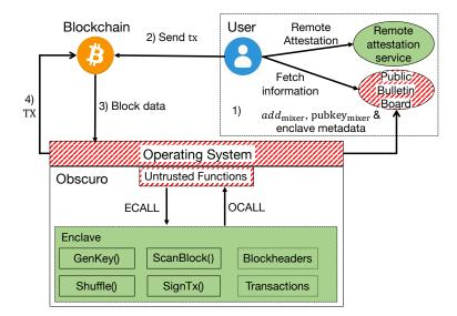
Figure 2: The OBSCURO architecture. Components in the green background are trusted, while the ones in the red stripe background are untrusted.
