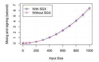
Figure 7: OBSCURO signing and mixing time with/without SGX.
