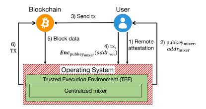
Figure 1: A baseline solution using a hardware-based trusted execution environment (TEE). Components in green background are trusted, while the ones in red stripped background are untrusted.
