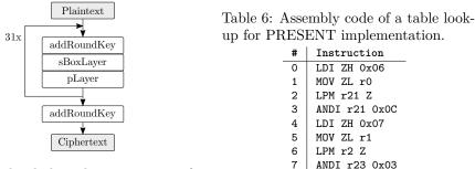
Figure 4: High-level algorithmic overview of PRESENT cipher.
