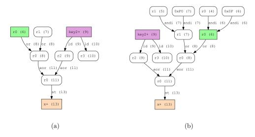
Figure 3: Subgraph constructed from node "r0 (6)" of data flow graph in Figure 2 with depth (a) 0 and (b) 1.
