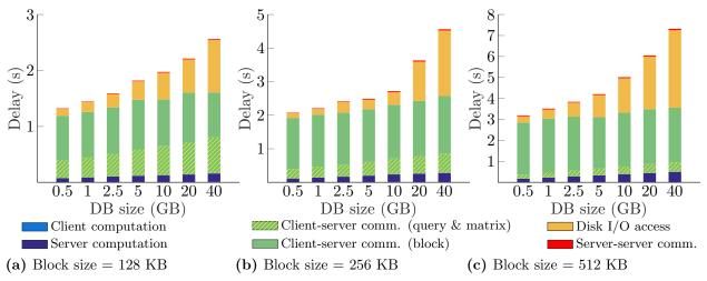
Figure 5: Detailed cost breakdown of S<sup>3</sup>ORAM on a laptop with home network.
