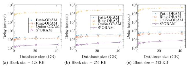
Figure 3: End-to-end delay of S<sup>3</sup>ORAM and its counterparts on a laptop with home network.
