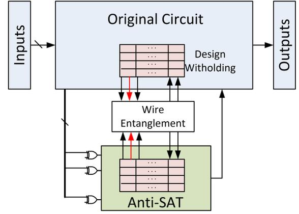
Fig. 7. Anti-SAT obfuscation based on design withholding and wire entanglement.
