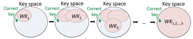
Fig. 3. Illustration of the iterative SAT attack process. Wrong key combinations are iteratively identified by a set of DIOs till no new ones exist.  $WK_i$  is the set of wrong key combinations identified by  $i$ -th DIO.
