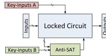
Fig. 2. A basic overview of Anti-SAT block enhanced logic locking.
