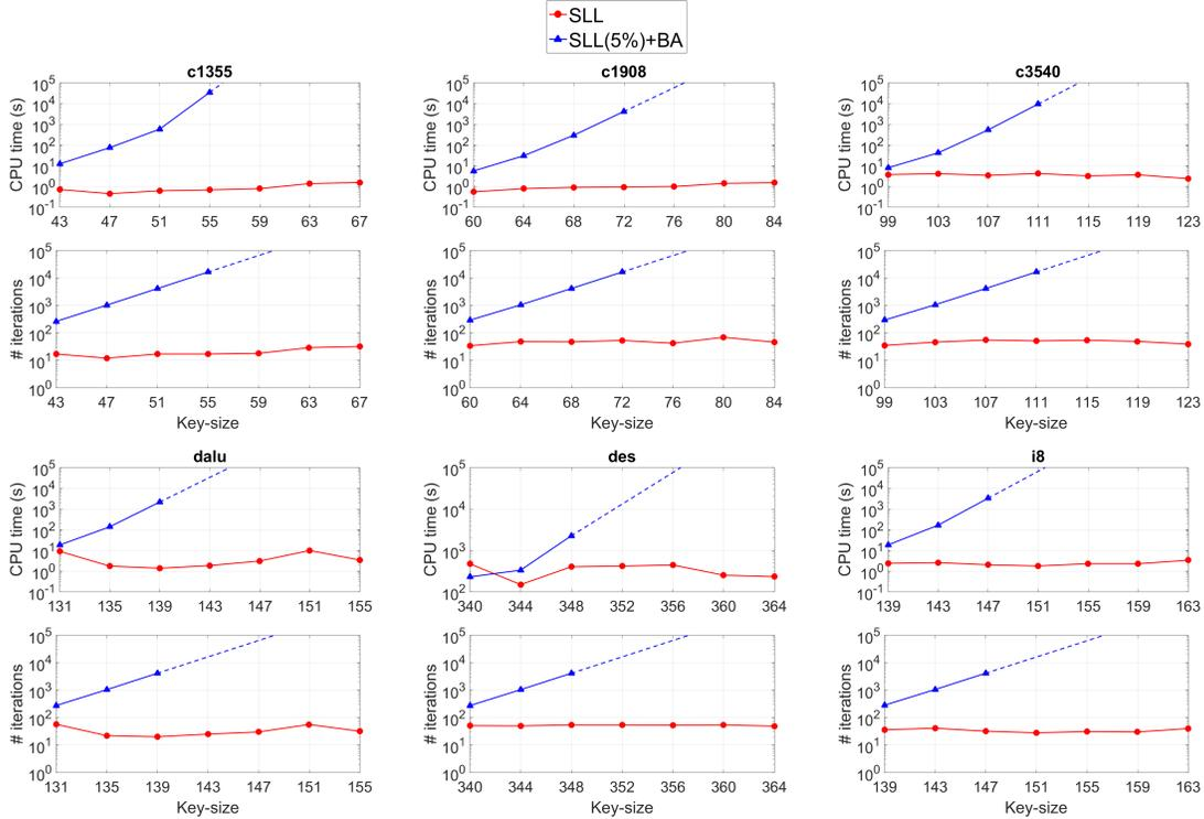
Fig. 10. SAT attack results on 6 benchmarks with three logic locking configurations: SLL and SLL(5%) +  $n$ -bit BA. Timeout is 10 hours ( $3.6 \times 10^4$  s). The dashed lines are the curve fitting results when the SAT attack has time-outed after certain key-size.
