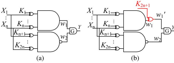
Fig. 5. Anti-SAT block design and obfuscation. (a) one possible construction of function  $g$  to ensure large number of SAT attack iterations; (b) an additional key-gate is inserted for functional obfuscation.
