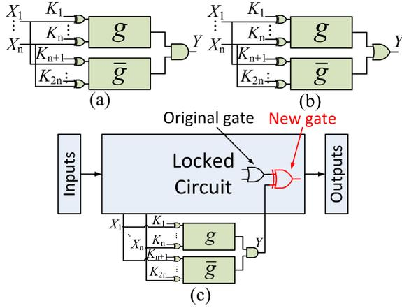
Fig. 4. Anti-SAT block configuration: (a) Type-0 Anti-SAT: always outputs 0 if key values are correct; (b) Type-1 Anti-SAT: always outputs 1 if key values are correct. (c) Integrating the Type-0 Anti-SAT block into a circuit.
