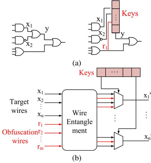
Fig. 6. Design withholding and entanglement technique: (a) design withholding and (b) wire entanglement.
