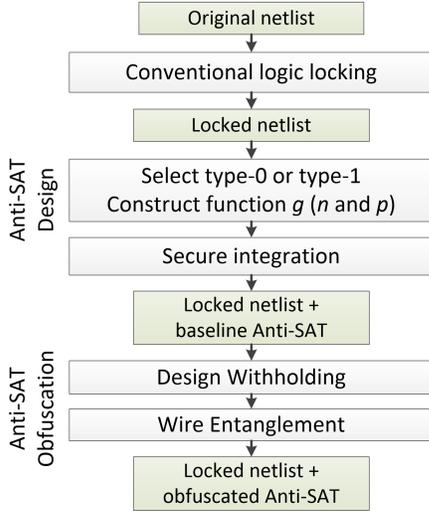
Fig. 9. Design flow of Anti-SAT based Logic Locking.
