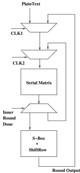
Fig. 1. Datapath Design of our Proposed Method
