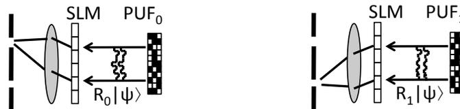
Figure 1: A single SLM configuration can verify  $q$  distinct responses. Example for  $q = 2$ .
