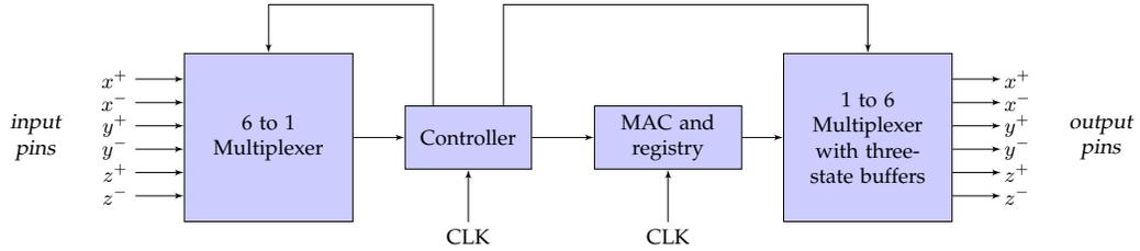
Fig. 15: Logic diagram of a 3D switch-box
