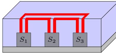
Fig. 19: Three switch-boxes embedded at substrate level with interconnections over the top layers
