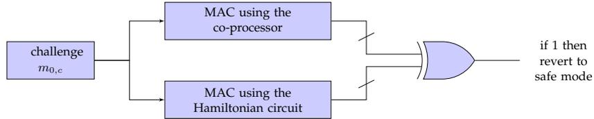
Fig. 18: Device integrity verification scheme
