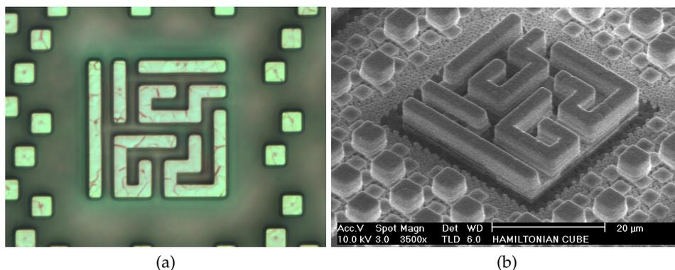
Fig. 13: Top layer view (a) and tilted SEM view (b) of a  $26\mu\text{m}$  wide  $6 \times 6 \times 6$  cage implemented in a 130nm technology ( $\times 2500$ )<sup>7</sup>
