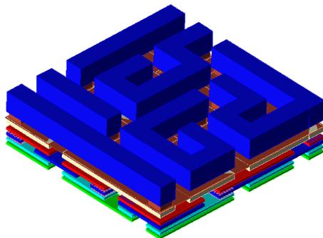
Fig. 12: 3D layout of a cage of size 6 (130nm, 6 Metal Layers Technology)
