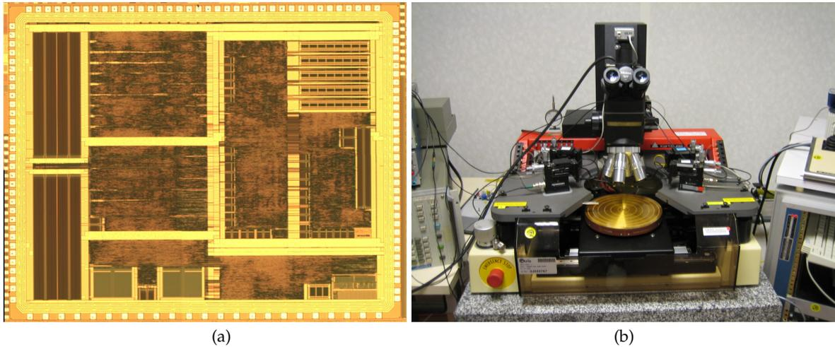
Fig. 22: A decapsulated chip with an exposed pad ring (a) and an optical probing station (b).
