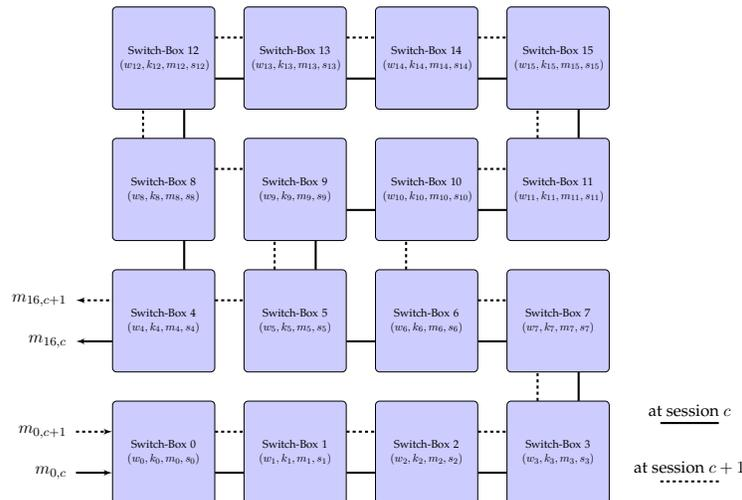
Fig. 17:  $4 \times 4$  dynamic switch-box grid routed at  $c$  and  $c + 1$  (illustration)
