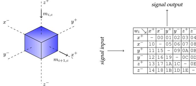
Fig. 14: Example of a 3D switch-box programmed with a routing configuration  $w_i = 0 \times 13$
