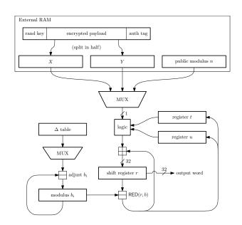
Figure 1. Simplified block diagram of a bit-serial BlueJay hardware implementation. Ciphertext  $C_i = C \bmod b_i$  is produced and transmitted one word at a time.
