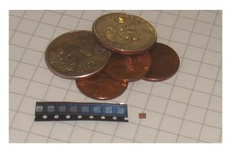
Figure 2. Implementations were compared on the Cortex M0 platform. Pictured is NXP LPC1102, a Cortex M0 self-contained system-on-chip (with an on-chip clock source) that has WLCSP16-packaged external surface area of  $2.17 \times 2.32 = 5.03 \text{ mm}^2$  or  $\frac{1}{128\text{th}}$  of a square inch.
