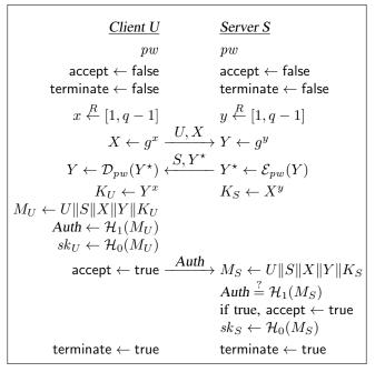
Figure 1. An execution of OEKE, run by client U and server S. The session key is  $sk = \mathcal{H}_0(U||S||X||Y||Y^x) = \mathcal{H}_0(U||S||X||Y||X^y)$ .
