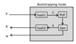
Figure 2: Bootstrapping mode. The control layer receives a pre-challenge P. The pre-challenge is hashed, yielding a challenge C, which is fed to the PUF. The PUF output is sent to the Gen function, which generates a secret key k and helper data w. The key k is hashed, yielding the response R. Finally, the control layer outputs the helper data w and the response R.
