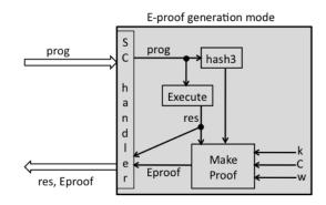
Figure 5: E-proof generation mode. The protocol is run through a SC. The SC-key in use is the hash of the secret key k; this k never leaves the CPUF. The user sends a program, which is executed and also hashed by the CPUF. The key k is used by the MakeProof function to certify the program hash, the result of the computation, and the SC setup parameters C, w.
