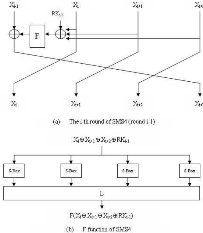
**Fig. 1.** Schematic Description of the SMS4 Round Function
