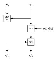
Fig. 2. The Threefish MIX operation.
