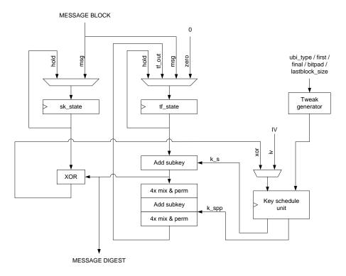
Fig. 4. Datapath of the Skein hardware module with eight unrolled Threefish rounds.
