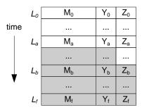
**Fig. 1.** Log file under delayed detection attack. Data in shaded area can be controlled by an attacker. *a*: time at which log entries are uploaded to T; *b*: break-in time; *f*: index value of last log entry as well as time when V receives a copy of log file from U.
